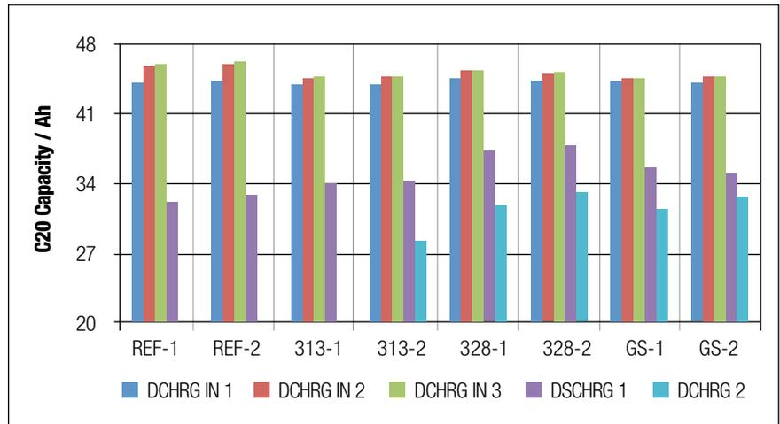
**Figure 3: The development of the C<sub>20</sub> capacity as cycling progresses.**
