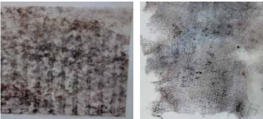
**Figure 6:** (a) the PET scrim after removal from the positive plate with its structure intact. (b) shows part of the glass scrim, removal was problematic as the fibres have lost their mutual cohesion
