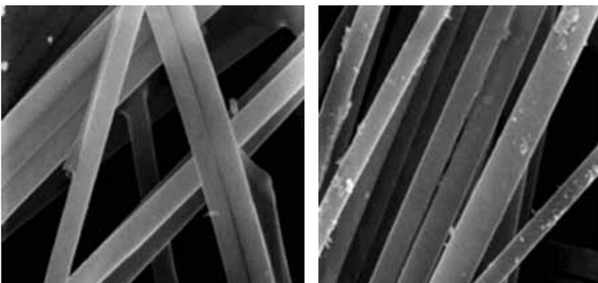
**Figure 8:** SEM image of the glass fibre scrim before (a) and after (b) testing, magnification 1000x
