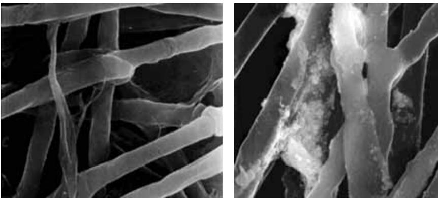
**Figure 7** (a) SEM image of the PET fibre side of Dynagrid® NG328 before use, (b) image of PET fibres' after discharge-charge cycling to end of battery life, magnification 500x
