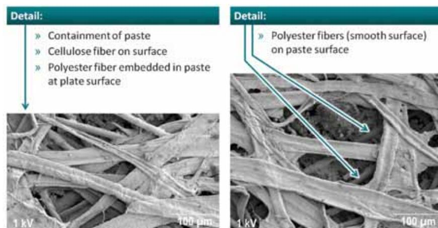
**Figure 2: Micrograph of Dynagrid® NG328 in position of lead plate**
