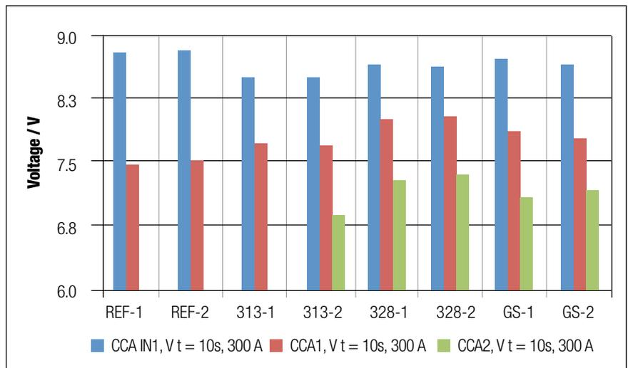
**Figure 4: Cold cranking ability, EN current**
