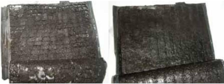
**Figure 5:** (a) Positive plate from the reference battery after removing the separator, shedding is clearly visible (b) Positive plate from Dynagrid® NG328 battery after removing separator, active mass is held in place with material loss through shedding being prevented.
