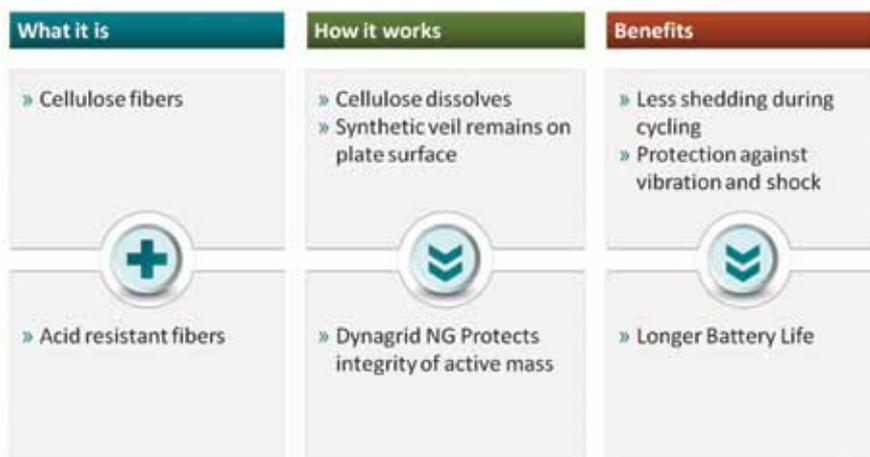
**Figure 1: Schematic overview of the manner in which the Dynagrid® NG328 extends battery cycle life**
